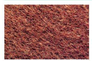
The TBM is a non-woven nylon fibre fabric uniformly impregnated with aluminium oxide or silicone carbide abrasive grains through the binding agent action of synthetic resins.
